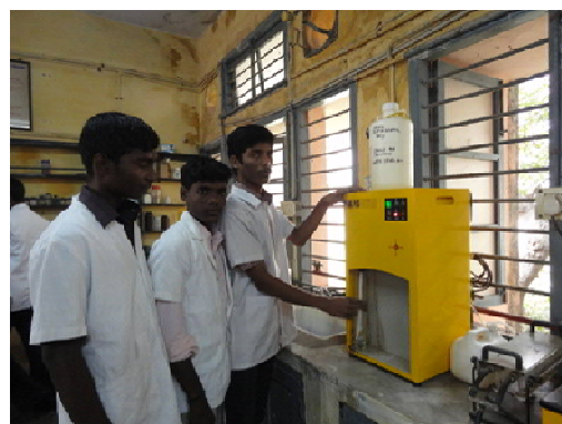
N Digester (FIST)
