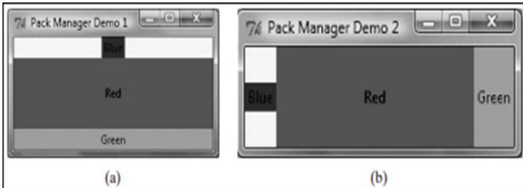
Fig. 6.2 (a) The pack manager uses the fill option to fill the container. (b) You can place widgets side by side.
