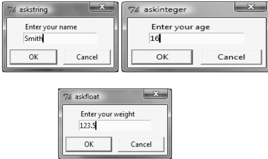
Fig 14.1 You can use the standard dialogs to display message boxes and accept input.
